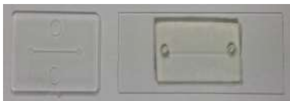
Fig.1. Microchips fabricated with PMMA and PDMS.
