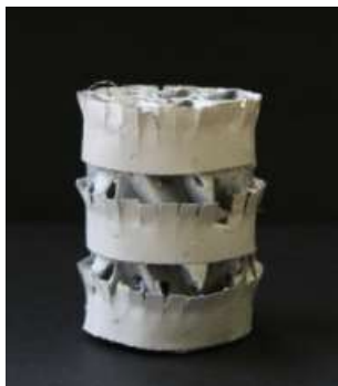
Fig. 2. Structured packing with silica-based coating containing lipase CALB.
